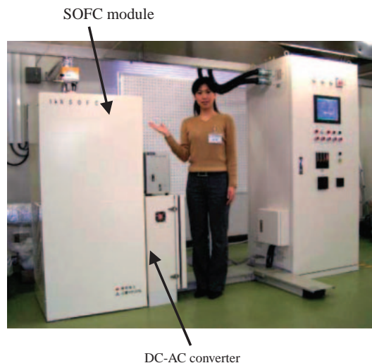
Fig. 20. SOFC system developed recently by Mitsubishi Materials by using LSGMC electrolyte.
